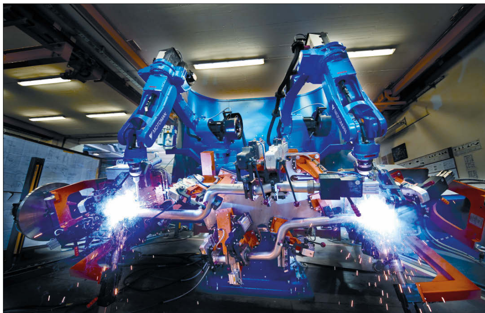
Picture 3. Welding robot cell
